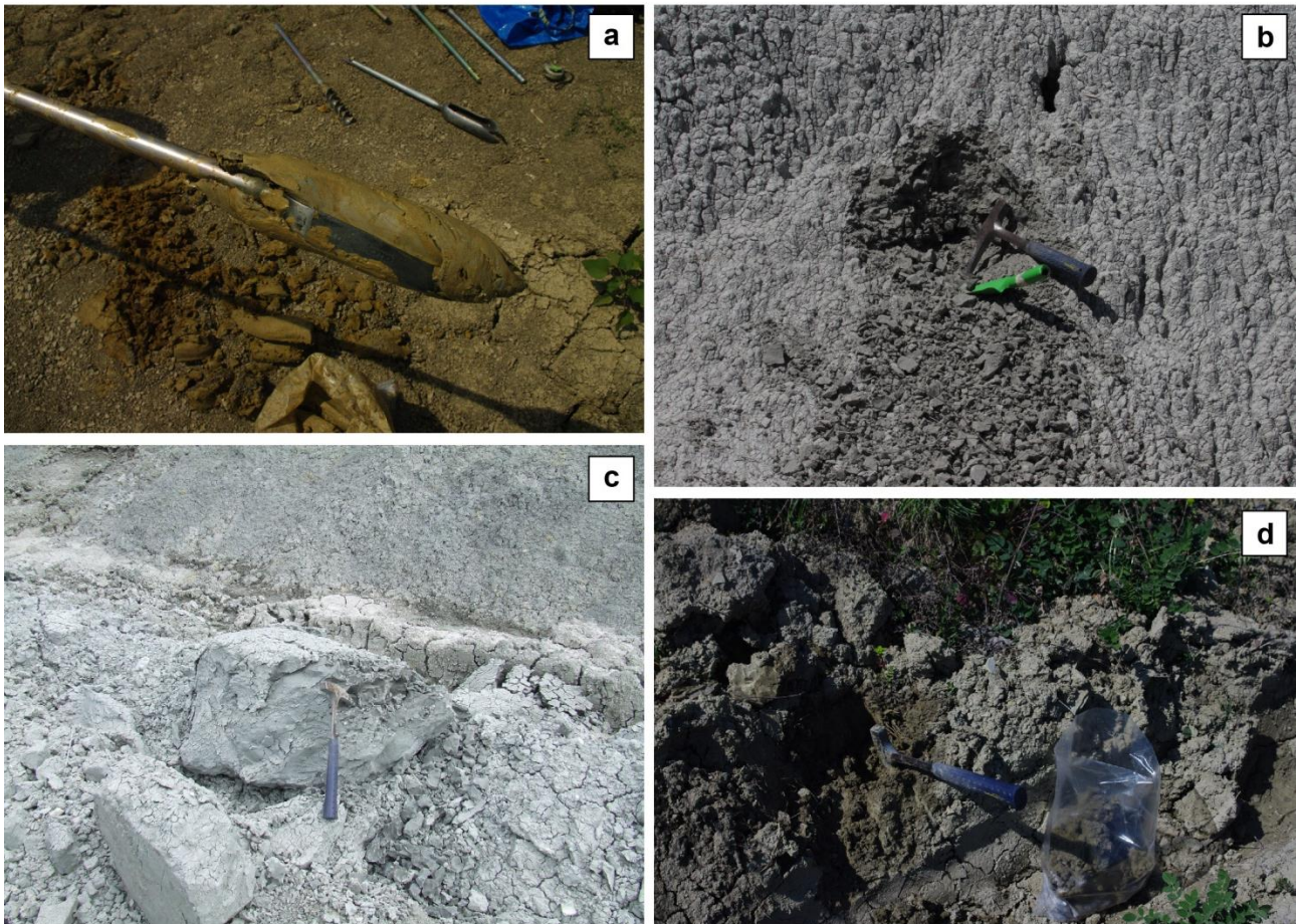
Fig. 3. Representative images showing the sampling of clay (a) via manual drilling, (b, c, d) directly on the outcrop.
